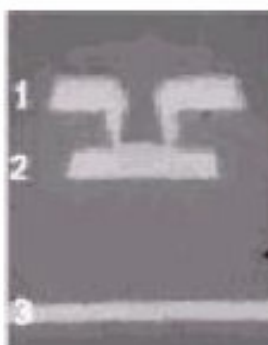
Figure 7: Microvia structure
